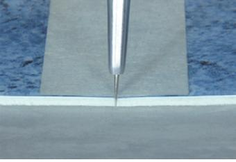
The patented needle system opens the seam area briefly and the cold-welding liquid runs along the needle into the whole cross section of the seam. The adjacent edges are moistened by the cold-welding liquid, temporarily dissolved and melted together, becoming strong and durable after a short period of time.
